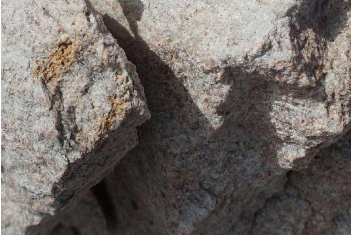
5: Closeup of previous picture (see arrow). The light grey to white rock is composed of 35 % quartz, 40 % feldspars, 20 % muscovite and 5 % opaque phases. The pink crystals are probably of potassium feldspar.
